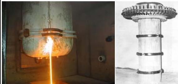
**VNIKhT.** H = 3.5 m, d = 650 mm, up to 2500°C (Ar, air, vacuum). **50 kg / h** of Fe-, Zr-, Nb-, U-alloy (Gotovchikov et al.).
